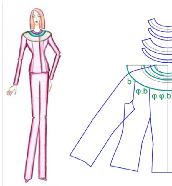
Figure 11. Applying of the golden ellipse fashion design and pattern making of a women’s jacket. CC BY Kazlacheva
