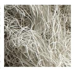
concentrated solution of the polymer is drawn through spinnerets at temperatures where the solvent evaporates.
